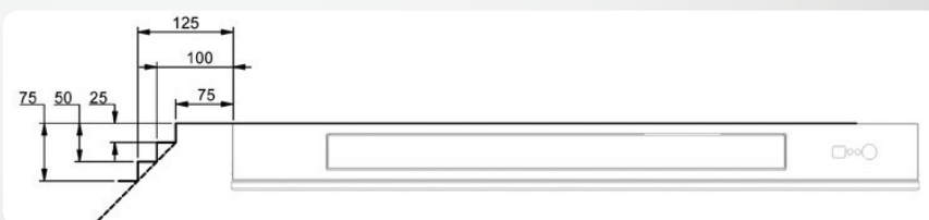
Arriva surround clearances
